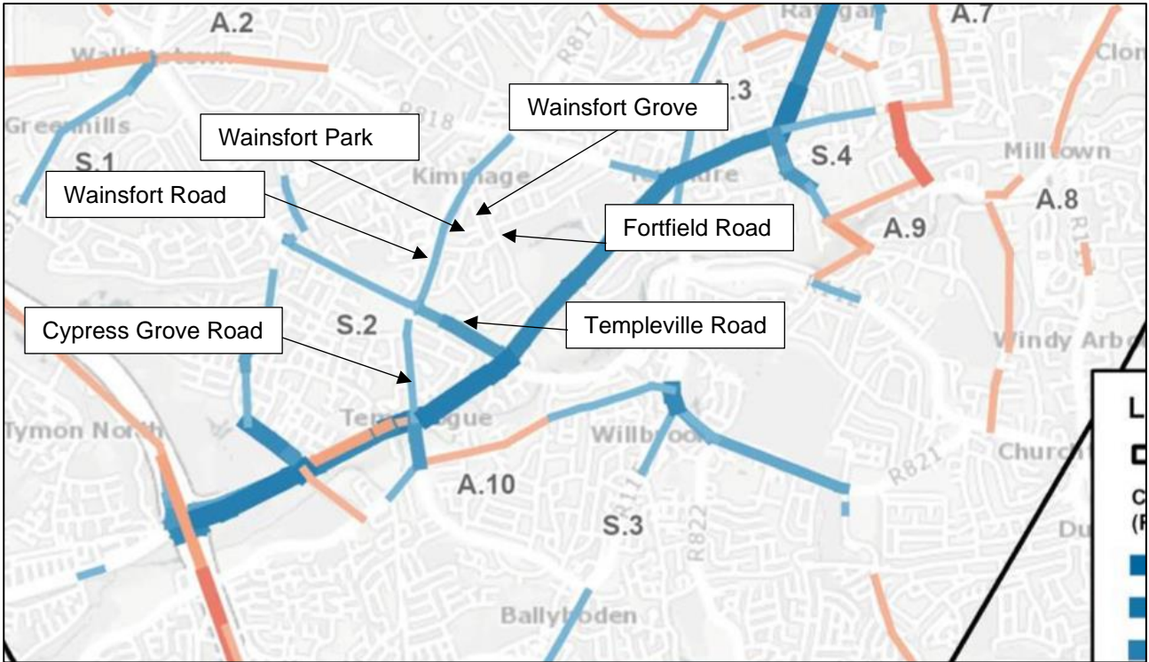
Figure 3.285.1 Flow Difference on Road Links (Do Minimum vs. Do Something), AM Peak Hour, 2028 Opening Year (Diagram 6.40 from Chapter 6 of the EIAR)
