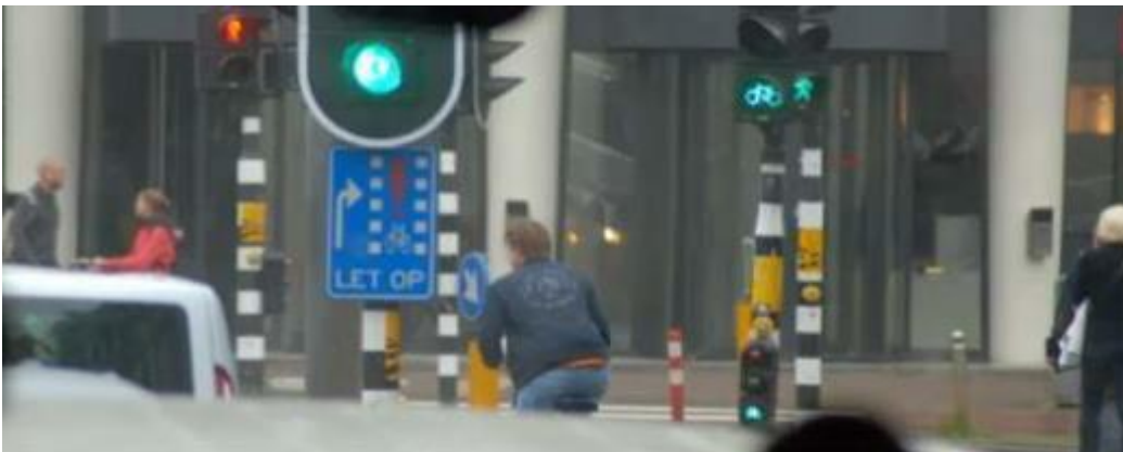
Figure 2.6.11 Example from the Netherlands of traffic signals + give way signage controlling turning traffic and cyclists (Source: Dutch Design Guide Ontwerpwijzer Fietsverkeer)
