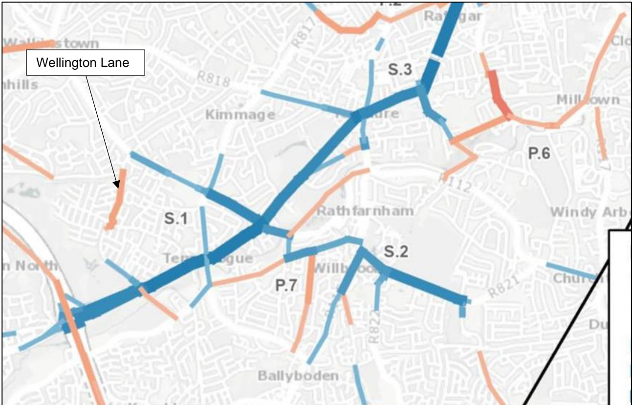
Figure 3.246.2 Flow Difference on Road Links (Do Minimum vs. Do Something), PM Peak Hour, 2028 Opening Year (Diagram 6.41 from Chapter 6 of the EIAR)
