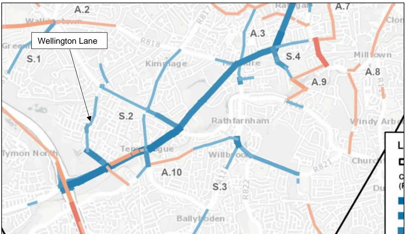
Figure 3.246.1 Flow Difference on Road Links (Do Minimum vs. Do Something), AM Peak Hour, 2028 Opening Year (Diagram 6.40 from Chapter 6 of the EIAR)
